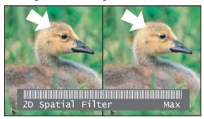
**2D filter set too high, seen a with split image**. (left image unprocessed). The finer details are lost.
